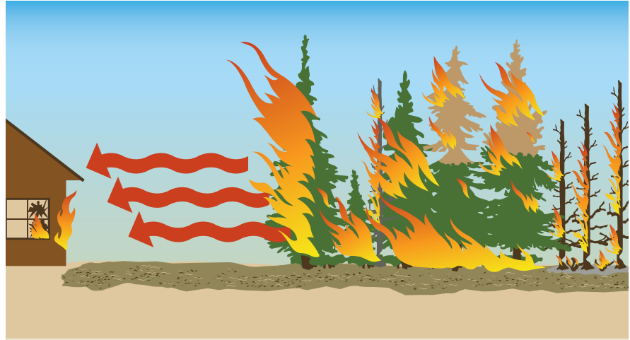
Figure 4-3. Radiant energy/heat transfers from burning trees to the side of the structure 30
