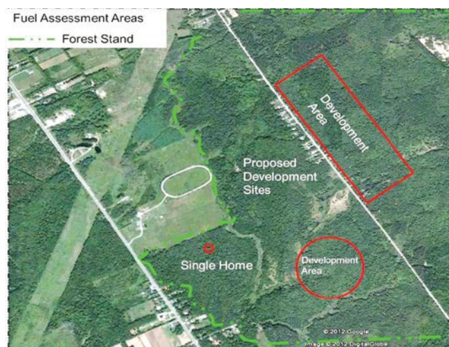
Figure 5-1. Proposed development within a forested area. The presence of hazardous forest types for wildland fire needs to be determined through wildland fire assessment. This assessment can be used to evaluate the merits of proposed development.
