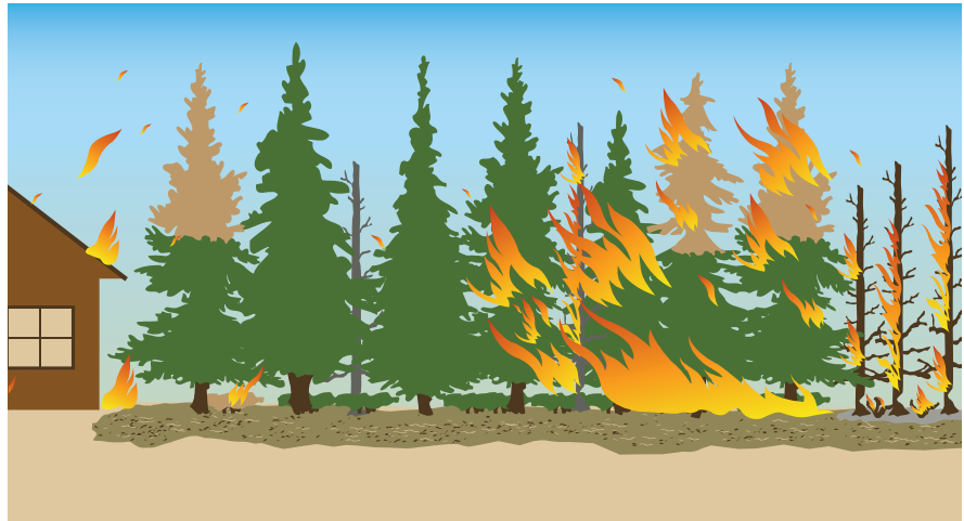
Figure 4-1. Effect of embers from the adjacent wildland fire landing on the roof of a structure and surrounding vegetation, resulting in further ignition of spot fires 25
