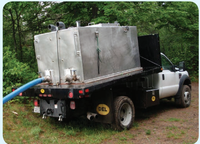
A 1-ton insulated multi-compartment truck
