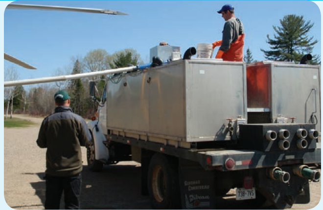
A 5-ton hatchery truck with insulated multi-compartment tanks
