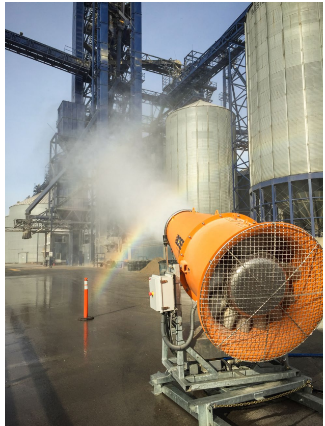
Figure 7. Atomized misting cannons, like the DustBoss unit pictured, are used in many industries to suppress fugitive dust. Source: BossTek, Peoria IL.
