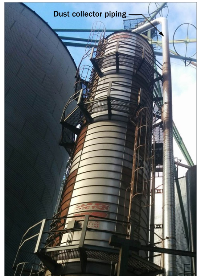
Figure 5. A tower dryer with dust control piping attached. Piping is connected to a cyclone filter to remove fines and red-dog from grain as it enters the top of the dryer.
