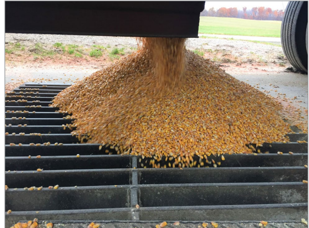
Figure 3. Reduce dust up to 90% by allowing grain to form a pile around the receiving grate as it is unloaded, known as “choke flow.”
