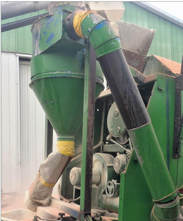
Figure 6. A cyclone separator, like the unit pictured on a grain cleaner system, uses rotational effects and gravity to remove particulate matter from an air stream.
