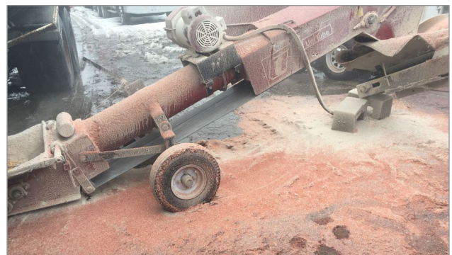
Figure 1. Grain dust known as “red dog” or “bees wings” is the most common particulate emission from grain-handling systems. It has a distinctive red-orange colour and can be produced in large quantities when handling corn.
