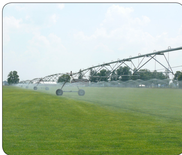
Figure 1. Irrigation of a sod farm using a lateral move irrigation system with low pressure spray nozzles.
