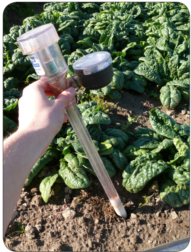
Figure 2. Measuring soil moisture with a tensiometer — a soil moisture gauge.
