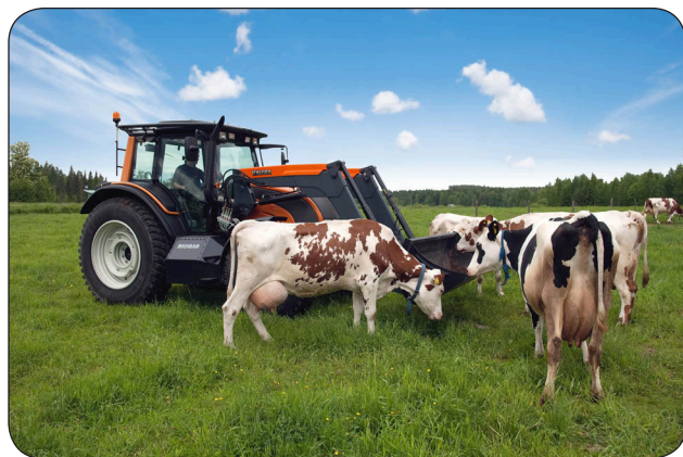
Figure 1. This Valtra tractor can operate for 3–4 hours on biogas between fill-ups. Photo courtesy of AGCO Valtra.
