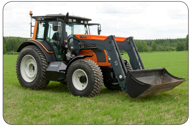
Figure 2. Dual-fuel tractor running on either diesel fuel or biogas. Photo courtesy of AGCO Valtra.
