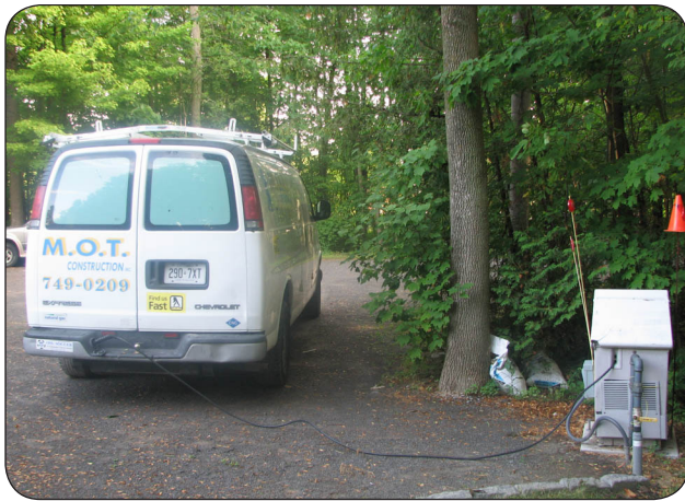
Figure 3. A commercial van being refuelled with natural gas. Photo courtesy of M.O.T Construction.
