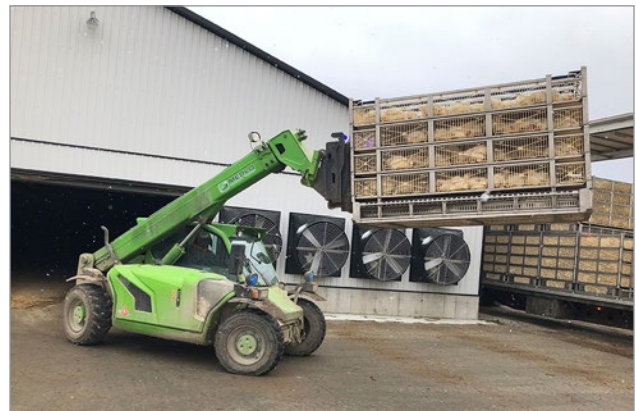
Figure 6. Merlo telehandler transporting a module.
