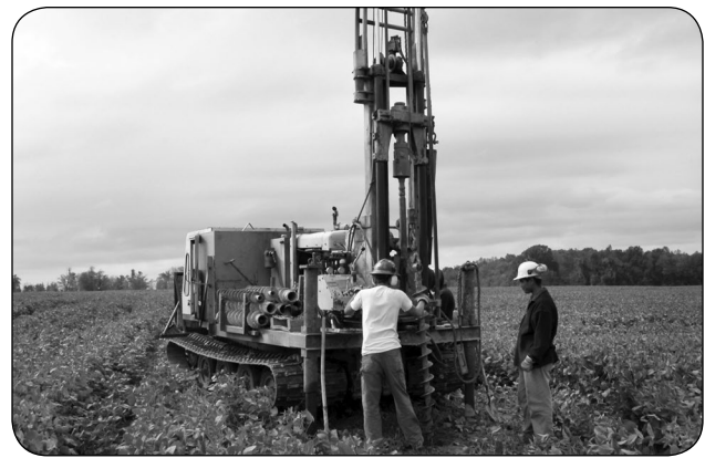
Figure 1. A mobile drilling rig is commonly used to take soil core samples for permeability testing.
