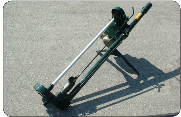
Figure 1. Vertical pump removed from tank.
