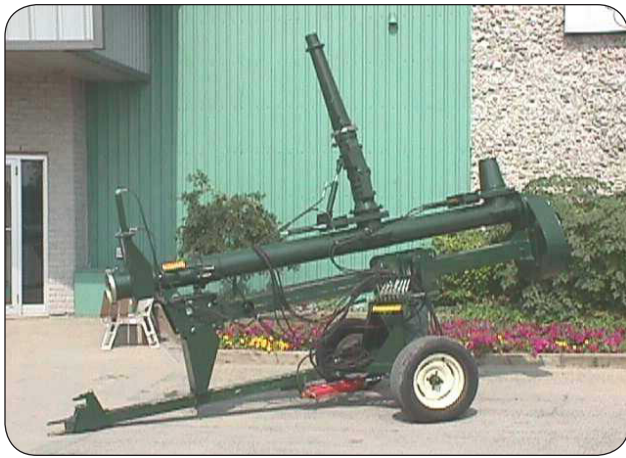
Figure 2. A vertical power take-off-driven pump in transport position.
