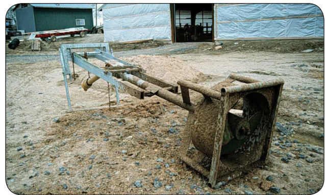
Figure 5. Propeller agitator used to circulate the manure in a raceway manure storage system.
