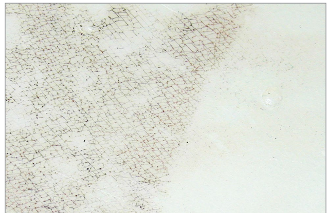
Figure 6. Poly tank showing evidence of crazing after coloured with a water-soluble marker.
