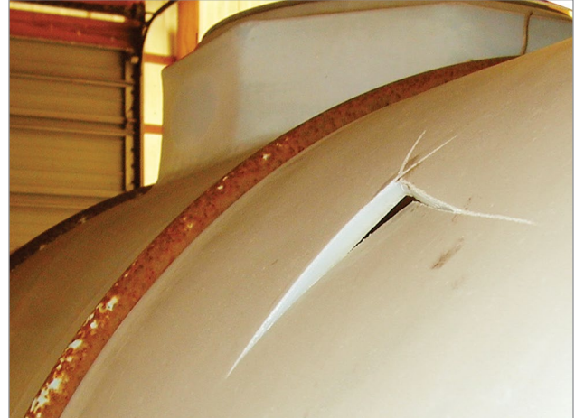
Figure 13. Upon being struck with a baseball bat to determine the tank integrity, this tank failed due to the brittleness of the plastic.
