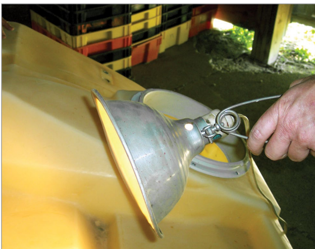
Figure 8. A bright light is used to candle the poly tank from the outside of the tank. Defects and cracks in the tank will show up as areas or lines of different light intensity (see Figures 9, 10 & 11).
