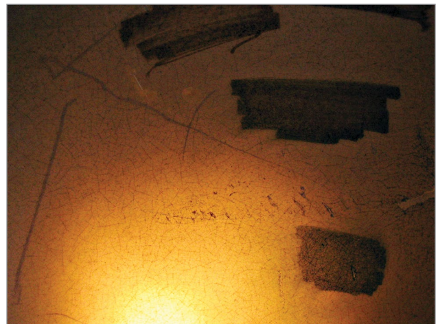
Figure 11. Candling reveals crazing of this tank.
