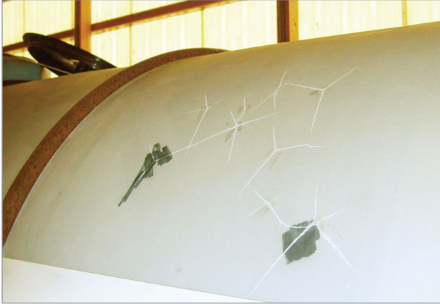
Figure 12. Tank showing signs of crazing and cracking when tested with a water soluble marker.
