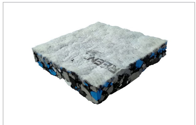
Figure 11. A permeable cover made of geotextile attached to recycled plastic foam.
