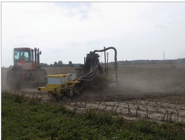
Figure 2. Using a drag hose for liquid manure application can minimize risk of soil compaction.
