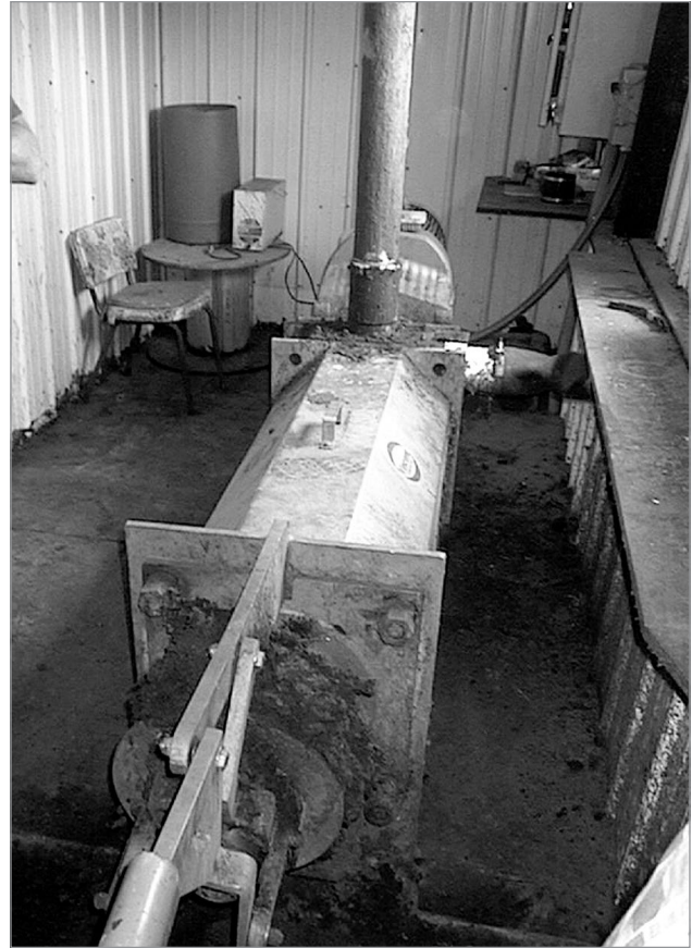
Figure 5. Screw separator extruding a solid material from liquid manure.
