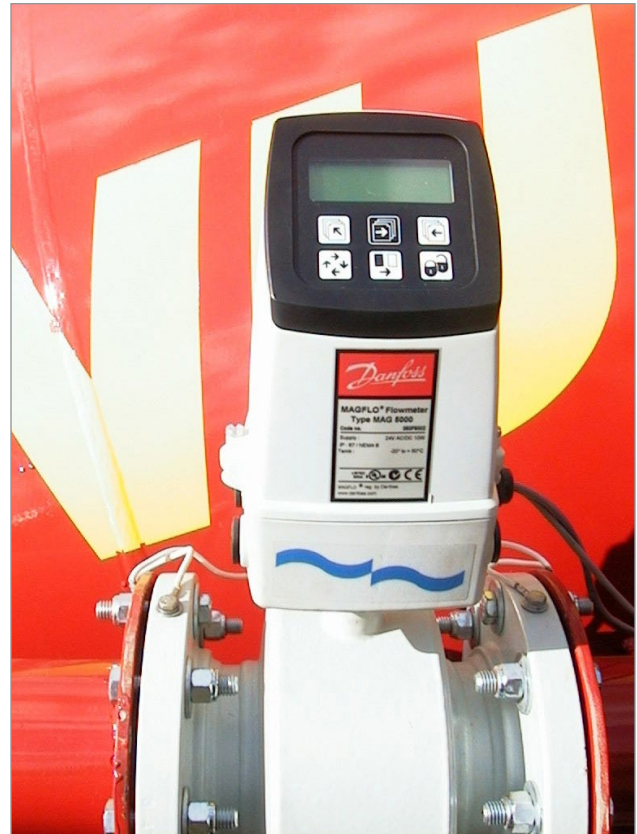
Figure 4. Example of a flow meter sensor mounted on a manure tanker. Talk to your local dealer for available products.
