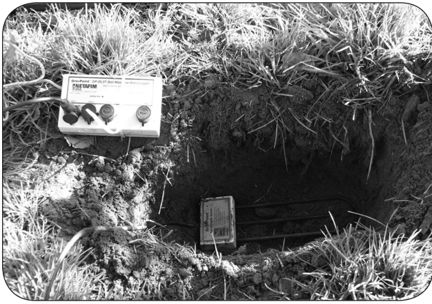
Figure 9. A TDR is positioned at the bottom of a hole, approximately 30 cm deep, in an apple orchard.
