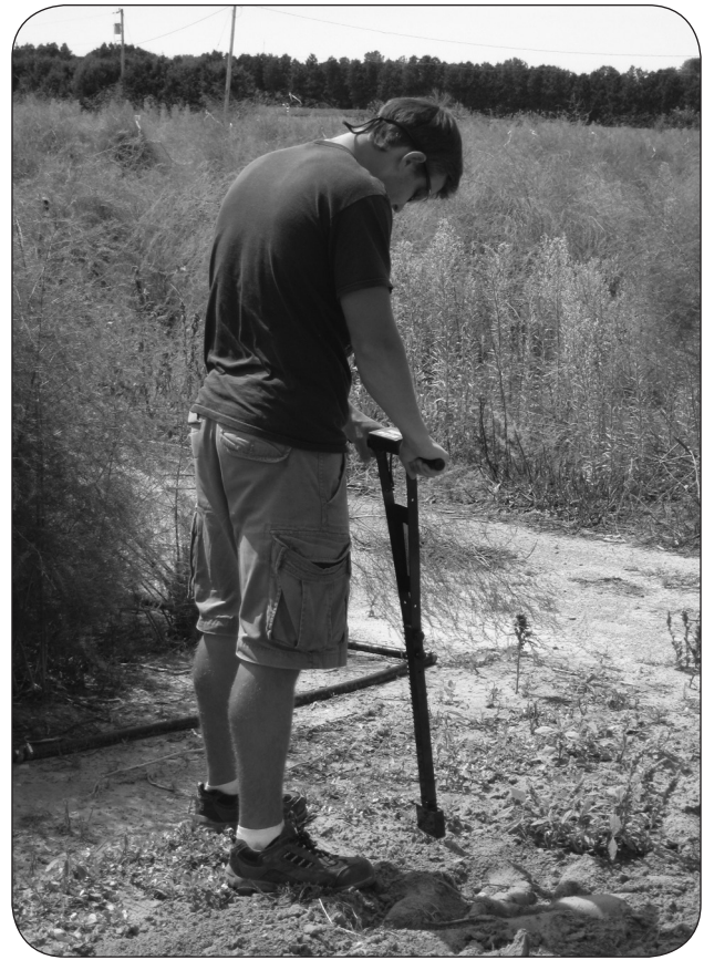
Figure 10. An irrigator pushes a TDR soil moisture probe attached to a waist-high insertion handle into the soil in an asparagus field. An instantaneous reading is taken and the probe is removed.
