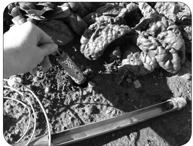
Figure 7. An electrical resistance block being inserted into a hole in the soil. Wires from a buried electrical resistance block are connected to a digital hand-held reader.
