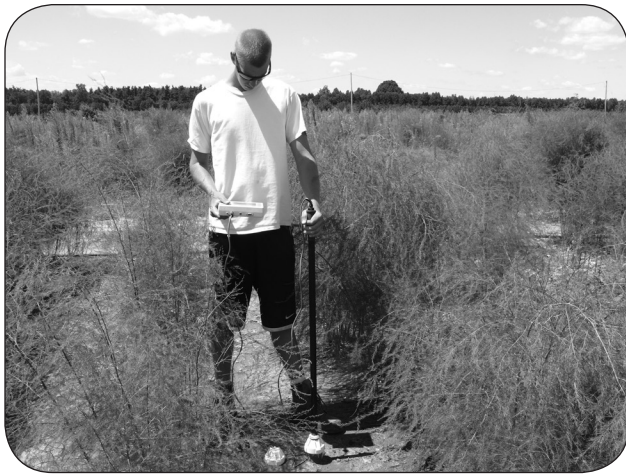
Figure 11. An irrigator lowers a capacitance probe with multiple monitoring depths into an access tube.
