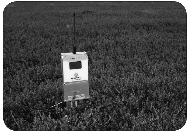
Figure 6. Digital tensiometer wirelessly transmitting data to a remote computer. Photo credit: Hortau Inc.
