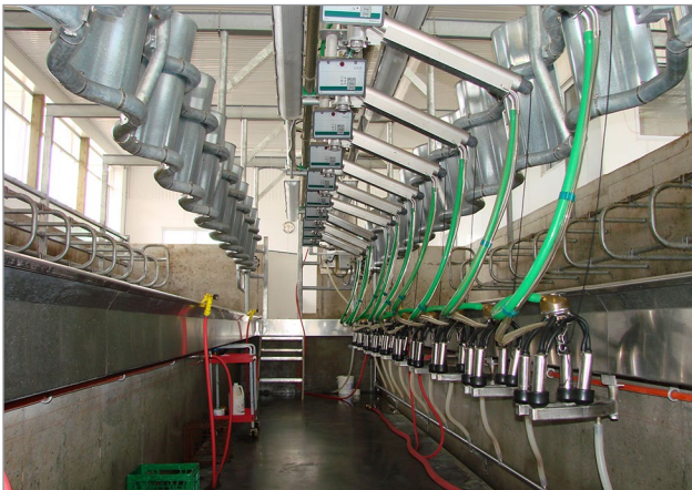
Figure 3. Rotating arms keep hoses out of the way.
