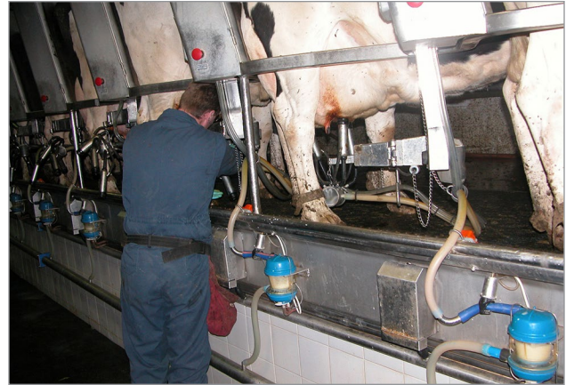
Figure 4. Sufficient pit depth allows milkers to attach equipment without strain.
