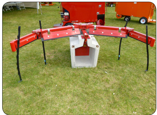
Figure 5. Display showing relationship between alley scraper and manure tube.
