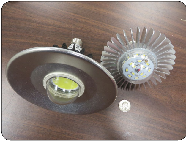
Figure 3. A hybrid LED bulb (right) showing the interior heat sink. Source: National Poultry Technology Center, Auburn University, www.poultryhouse.com .
