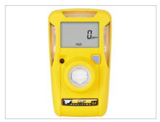
**Figure 1.** Example of a personal H<sub>2</sub>S gas monitor. This unit has a 2-year continuous use lifespan. Source: ITM Instruments Inc.
