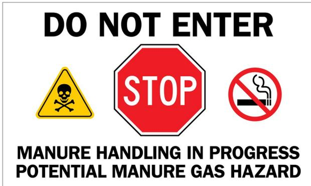
**Figure 2.** Sample warning sign posted during manure agitation.
