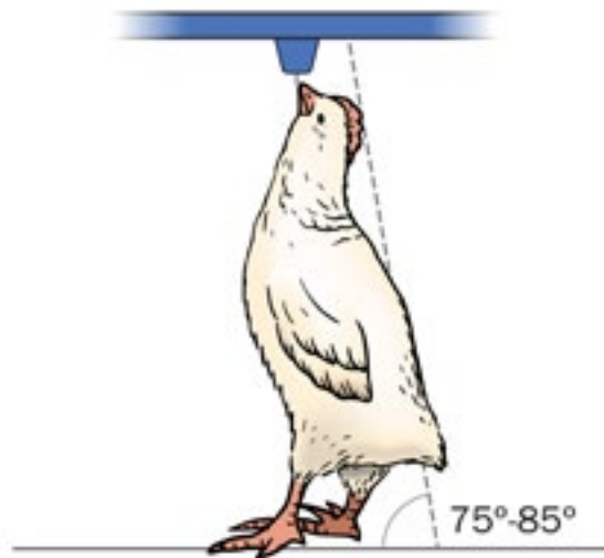
Figure 10. The proper height of a water nipple drinker for older birds.
