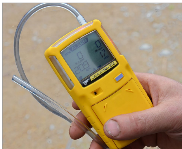
Figure 2. Example of handheld multi-gas detector used to monitor concentration of oxygen, hydrogen sulphide and explosive gas (% LEL means lower explosive limit), available at safety supply stores.
