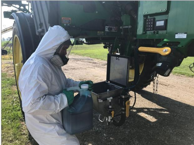
**Figure 3.** Use proper personal protective equipment (PPE) when handling pesticides. This sprayer includes a ground-level mixing station to allow easy pesticide loading while minimizing the risk of spills.
