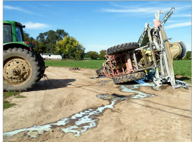
**Figure 2.** This sprayer operator took a tight turn too quickly on soft ground with a full tank, resulting in equipment damage and a pesticide spill.
