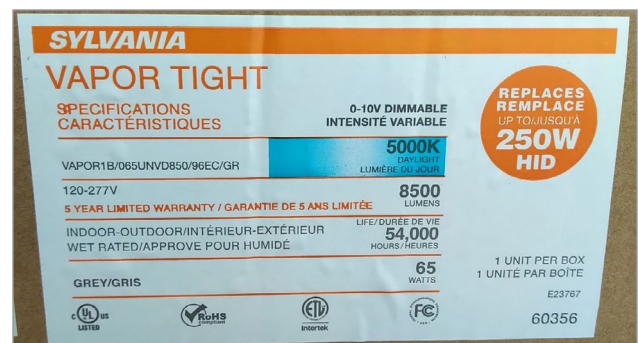
Figure 1. Typical information available on light fixture packaging. This is an 8-foot-long linear LED fixture in a wet rated, vapour-tight enclosure.
