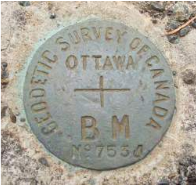
Figure A2-6. A geodetic survey benchmark.
