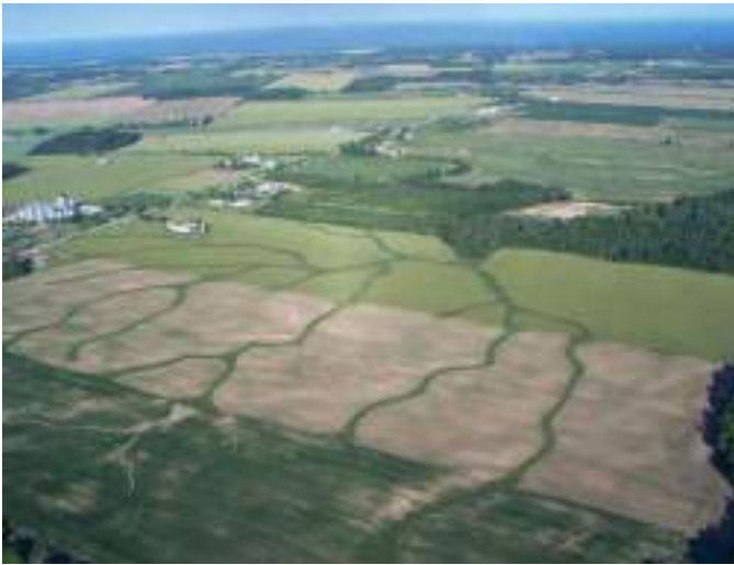
Figure B4-14. Aerial view of grassed waterways. Source: Ausable Bayfield Conservation Authority, Ontario
