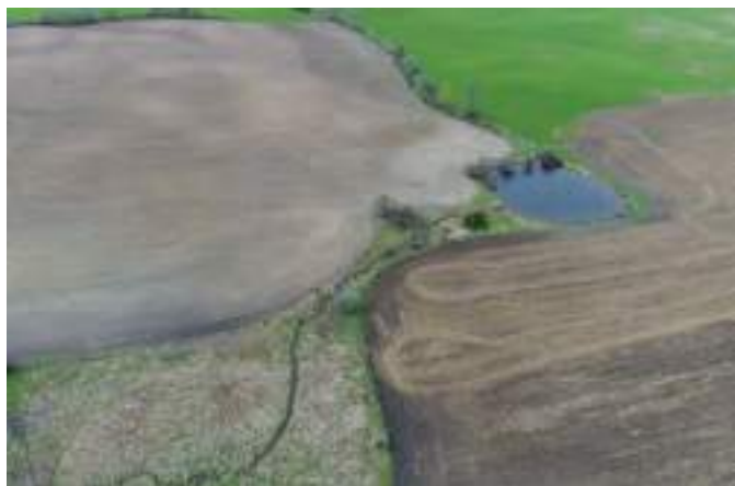
Figure B4-39. A wet pond always contains water. Source: Dietrich Engineering Ltd., Kitchener, Ontario
