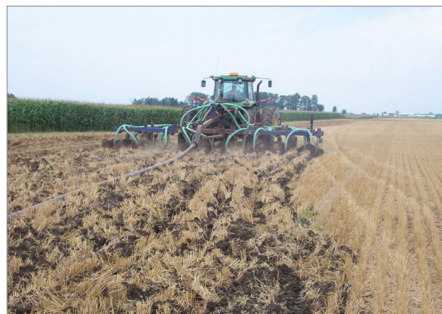
Figure 3. Liquid biosolids being land-applied using a drag hose.
