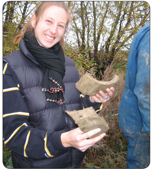
Figure 7. Example of sufficient clay for lining a reservoir.
