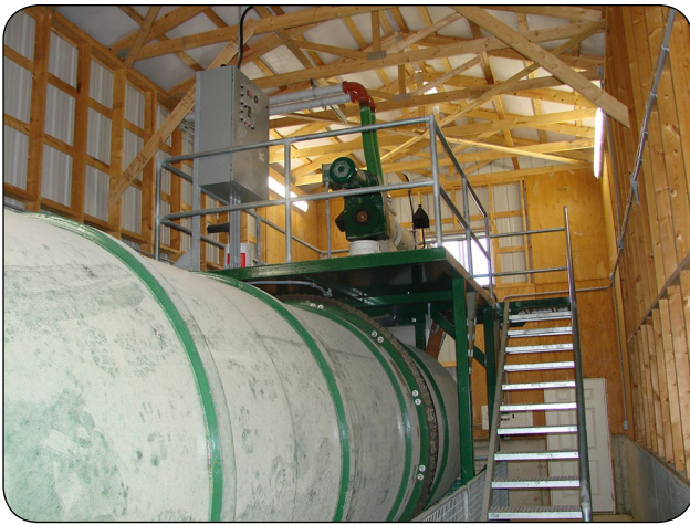
Figure 3. Drum composters accelerate the composting process.
