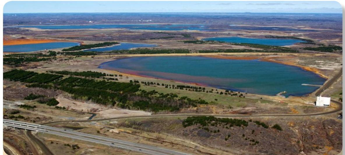
**View 3:** Aerial view of tailings ponds north of Regional Road 55 (lower left). Oxidation of the iron-bearing tailings produces rusty-coloured shorelines. The slopes of the tailings pond hills have been planted with trees and grasses. *Photo courtesy of the Ontario Geological Survey.*
