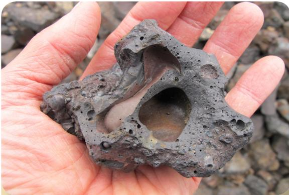
**View 6:** Fragment of slag displays a "Swiss cheese" texture that reflects its origin in a smelter furnace, where gas bubbles in molten slag were trapped as the slag began to cool to solid. Crushed slag is used as fill for the beds of roadways and railways in the Greater Sudbury area.
