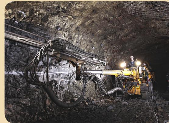
**View 2:** A rock-drilling machine used in an underground mine in Greater Sudbury. Drills mounted on the long mechanical arm are used to create holes that are then loaded with explosives. Blasting breaks the ore into rock fragments that are transported to surface and then to the mill for crushing and grinding.
