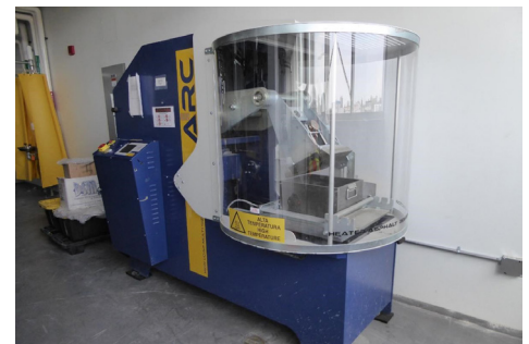
Bituminous slab compactor is used to produce representative sample slabs of several dimensions of bituminous mixtures laid and compacted on site.
