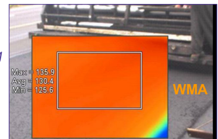
Figure 1b: Warm Mix Asphalt thermal image showing temperature ranges from a minimum temperature of 125.6°C to maximum 135.9°C, averaging 130.4°C.
