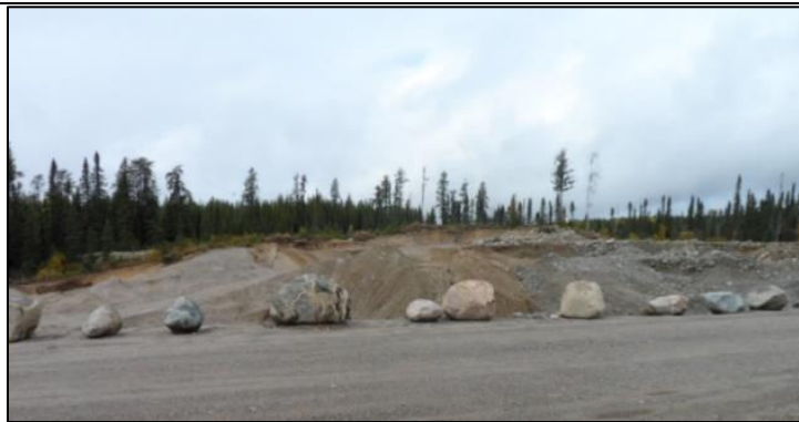
Picture #3: Pit 594L – Active pit with partial access controls(boulders) in place along the road to limit access to the pit and as a safety measure. This practice, auditors were told, is a safety hazard.
