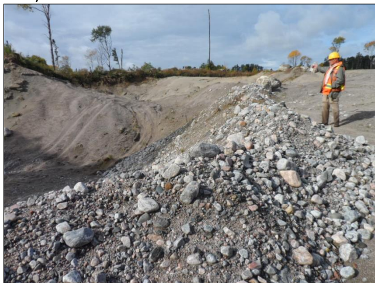
Picture #4: Pit 1306 L – An active aggregate pit with partial access controls – note how the berm does not completely bar access – also shows the pit surface is below the ditch line and is not sloped to 2:1 as required. This pit is a safety hazard.
