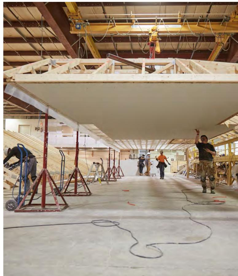
Image 10: Workers in a factory preparing different parts of roof structures.
