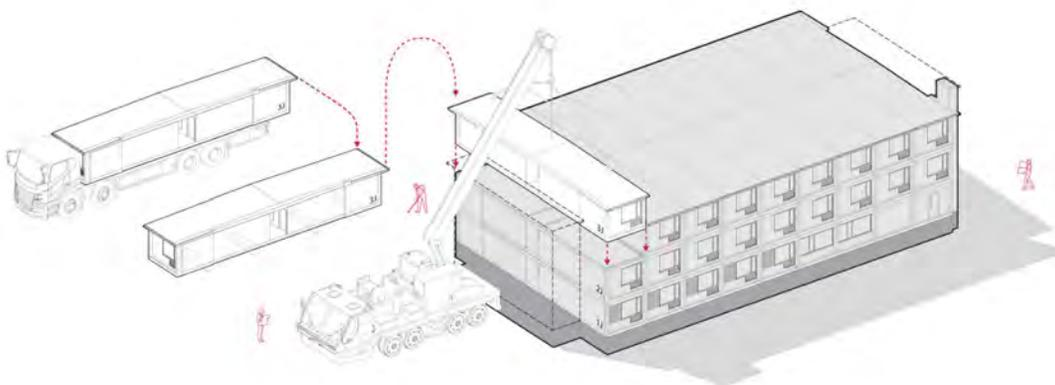
Diagram 3: A diagram illustrating the rapid assembly process of multi-residential modular housing. Image by Montgomery Sisam.
