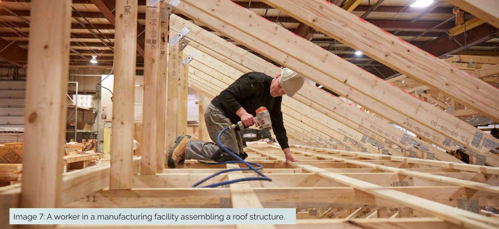
Image 7: A worker in a manufacturing facility assembling a roof structure.
