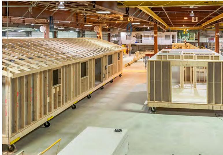
Image 11: Two partially completed modules in a manufacturing facility.
