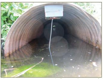
Photo 66. Camera securely fastened to top of culvert; note difficult to capture animals when water in culvert or tunnel. © K. Gunson
