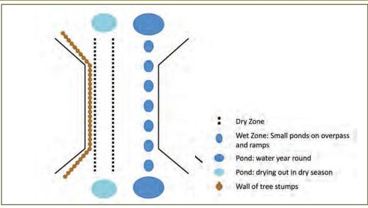
**Figure 2:** Example of a series of pools created along one side of an overpass (50 m long x 65 m wide). Amphibian passage was at least 1.5 times higher through the wetland zone than the dry zone. Adapted from van der Grift et al. 2009
