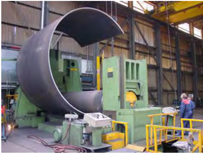
a) Pile rolling – credit SIF
