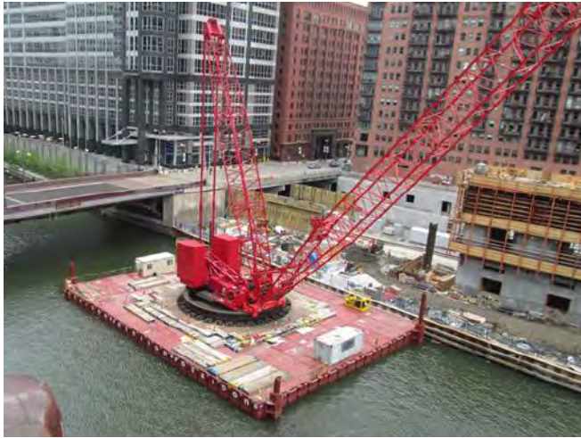
c) Poseidon portable sectional barge with spud-leg stabilisation, in use with a Manitowoc ringer mobile crane
