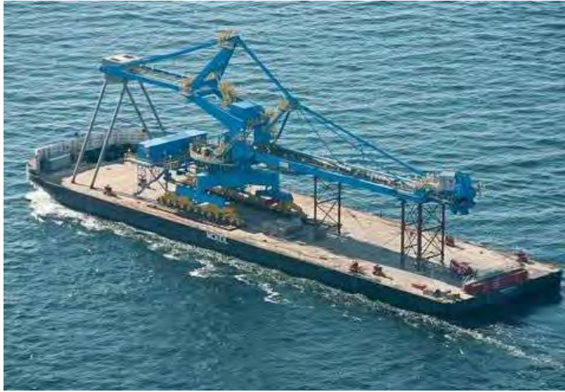
McKeil's "Nunavut Spirit", 32 m beam, 122 m (400 ft) length, spud legs for 30 m water depth.
