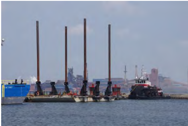
a) McKeil's "Jack-up 600", monohull with up to 6 legs
