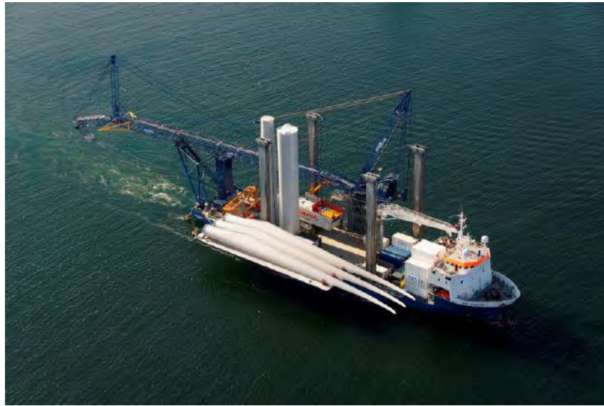
Figure 5-18 Sea Power leg-stabilized vessel
