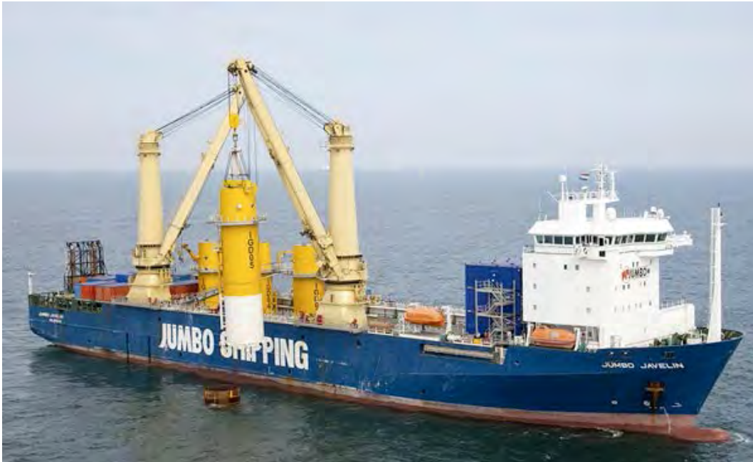
Figure 5-39 TP installation from heavy lift cargo vessel
