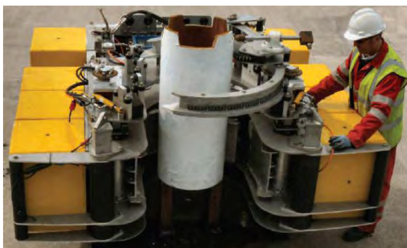
c) External cutting track and ROV manipulator
