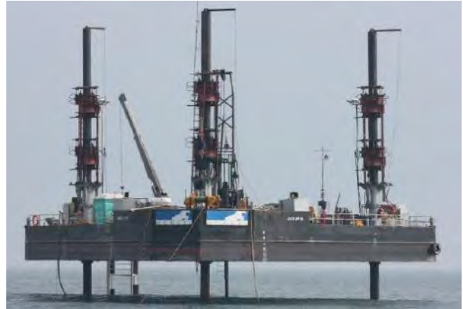
b) McKeil's "Jack-up 50", monohull with 4 legs
