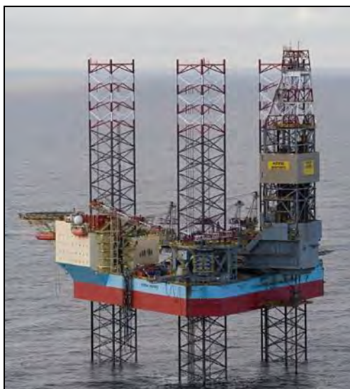
Figure 3-3 Typical modern jack-up drilling rig
