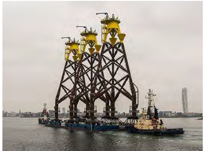
b) Baltic 2 jackets, 3-legged – credit Blue Water Shipping
