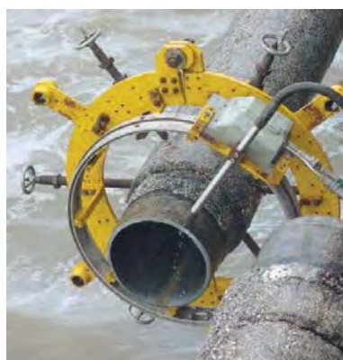
a) External cutting frame
