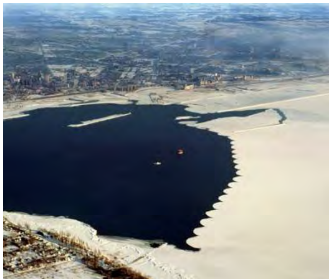
Figure 3-28 Ice boom at mouth of Niagara River, Lake Erie
