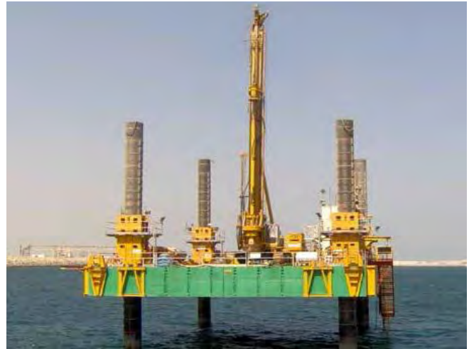
d) Combifloat (Flexifloat) modular floating and self-elevating platform
