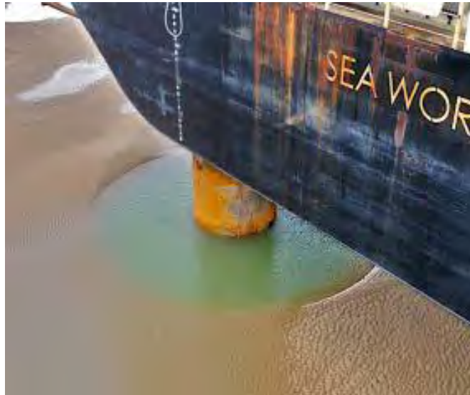
Figure 2-26 Scour hole around a jack-up leg
