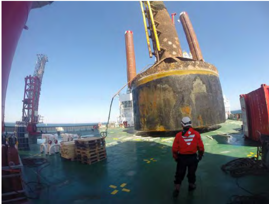
Figure 5-52 Lifting out of Horns Rev II met mast bucket foundation
