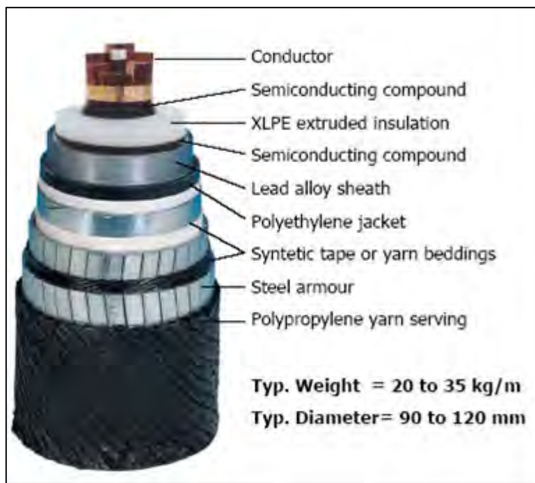
Figure 2-21 Components of a HVDC export cable
