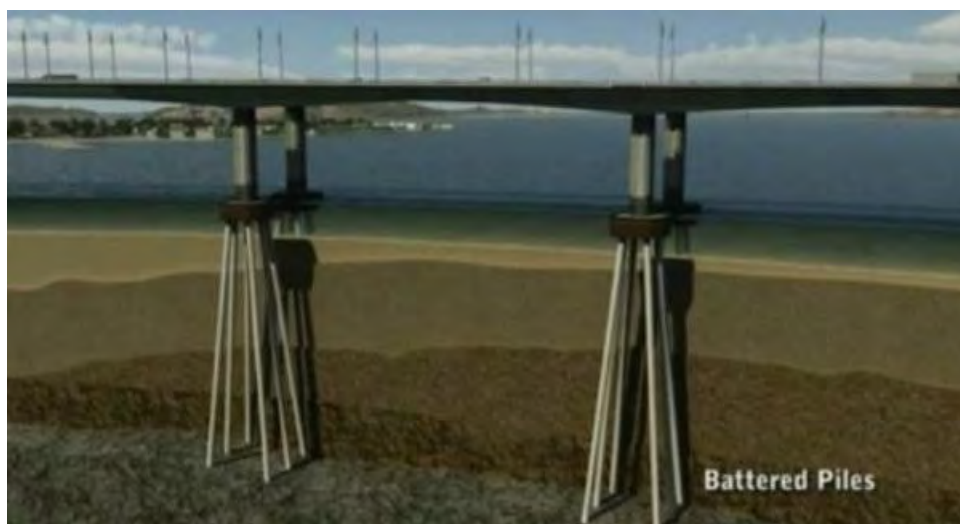
Figure 3-16 Angled or “battered” piles
