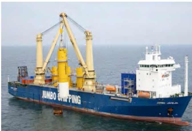
c) DP HLCV “Jumbo Javelin” installing TPs. 26.7 m beam, 144.21 m length, 2 x 900 te cranes, 17 kts transit speed
