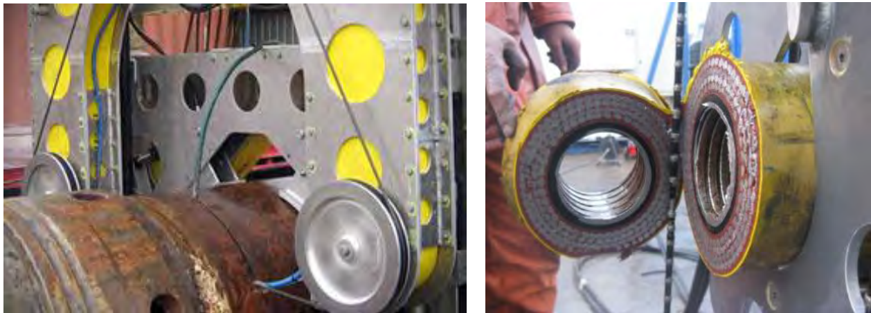
Figure 5-22 Diamond wire cutting
