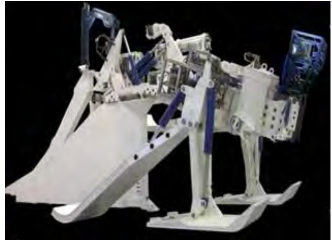
Cable plough on sleds
