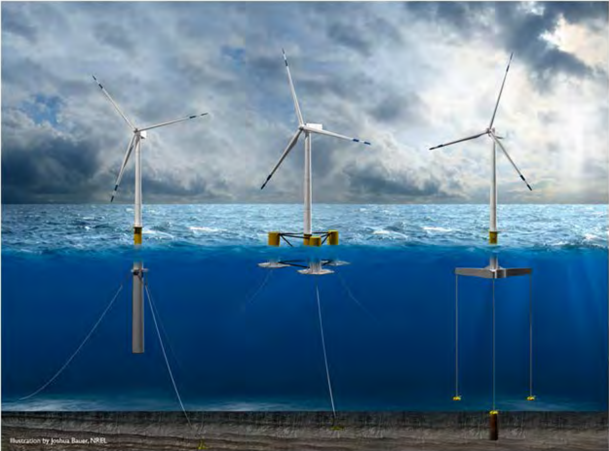
Figure 2-19 Floating support structure concepts
