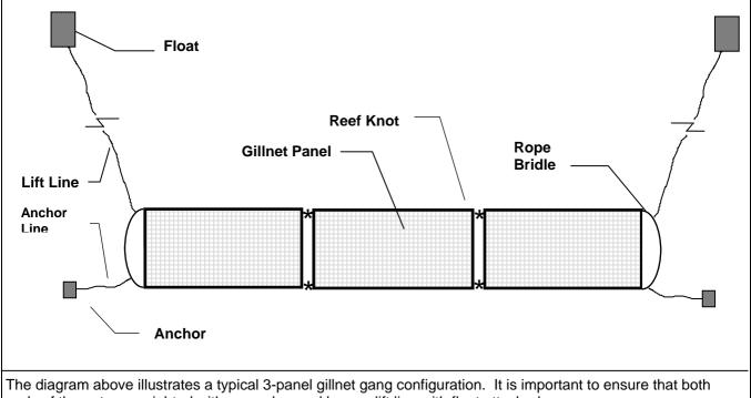
The diagram above illustrates a typical 3-panel gillnet gang configuration. It is important to ensure that both ends of the net are weighted with an anchor and have a lift line with float attached.
